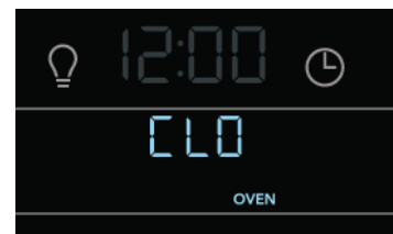
Figure 34: Message of open door that must be closed before oven can begin the clean cycle
