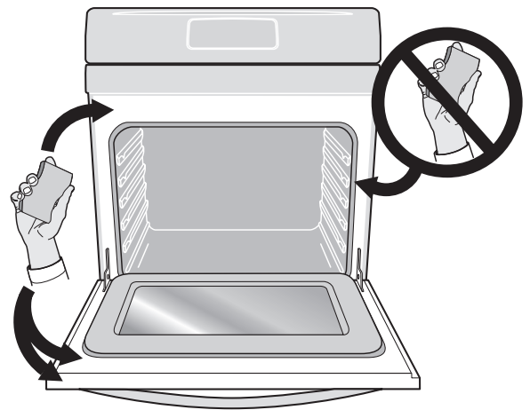
Figure 7: Clean around the oven door gasket
