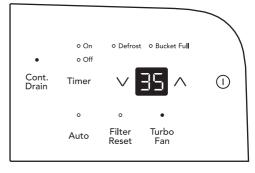
5. After a few days when the Relative Humidity has declined, press the Cont. Drain button to deactivate the Cont. Drain feature then press the HUMIDITY ∨ or ∧ buttons to choose a value between 35% to 85%, so the room is kept at a comfortable humidity. Pressing the ∨ or ∧ buttons will change the humidity selection in 5% increments. After you have set the desired humidity, the readout will display the actual room humidity.
