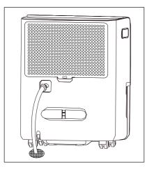
Select the desired humidity setting and fan speed on the unit for continuous draining to start.
