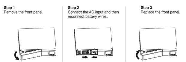
This UPS can be either placed on a desktop, mounted in a rack or installed in an upright position. Define the proper display orientation based on the configuration chosen to install this UPS.
