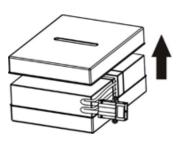
**Step 7**Replace the front panel of the UPS.
