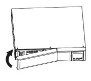
**Step 5**When done, replace the cover of the battery compartment and
