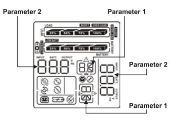
Two parameters need to be configured in order to set up the UPS. Refer to the following diagram.
