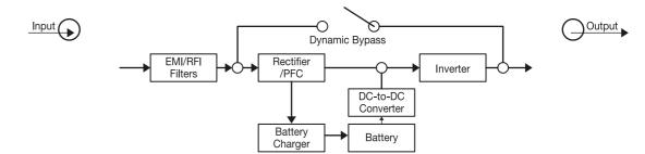
The UPS is composed of mains input, EMI/RFI filters, rectifier/PFC, inverter, battery charger, DC-to-DC converter, battery, dynamic bypass and UPS output.
