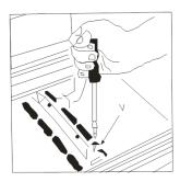
Unscrew the burner nozzle from the oven using the special nozzle wrench, or a 7 mm socket wrench, and replace it with a suitable nozzle for the new type of gas.
