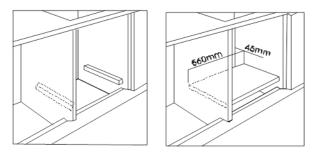
The panels of adjacent cabinets should be made of heat resistant material. In particular, cabinets with outer sheet must be assembled with glues with glues that can withstand temperatures of up to 100.
