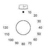
The minute hand can be used independently of the oven cooking function for a period of up to 120 minutes.
